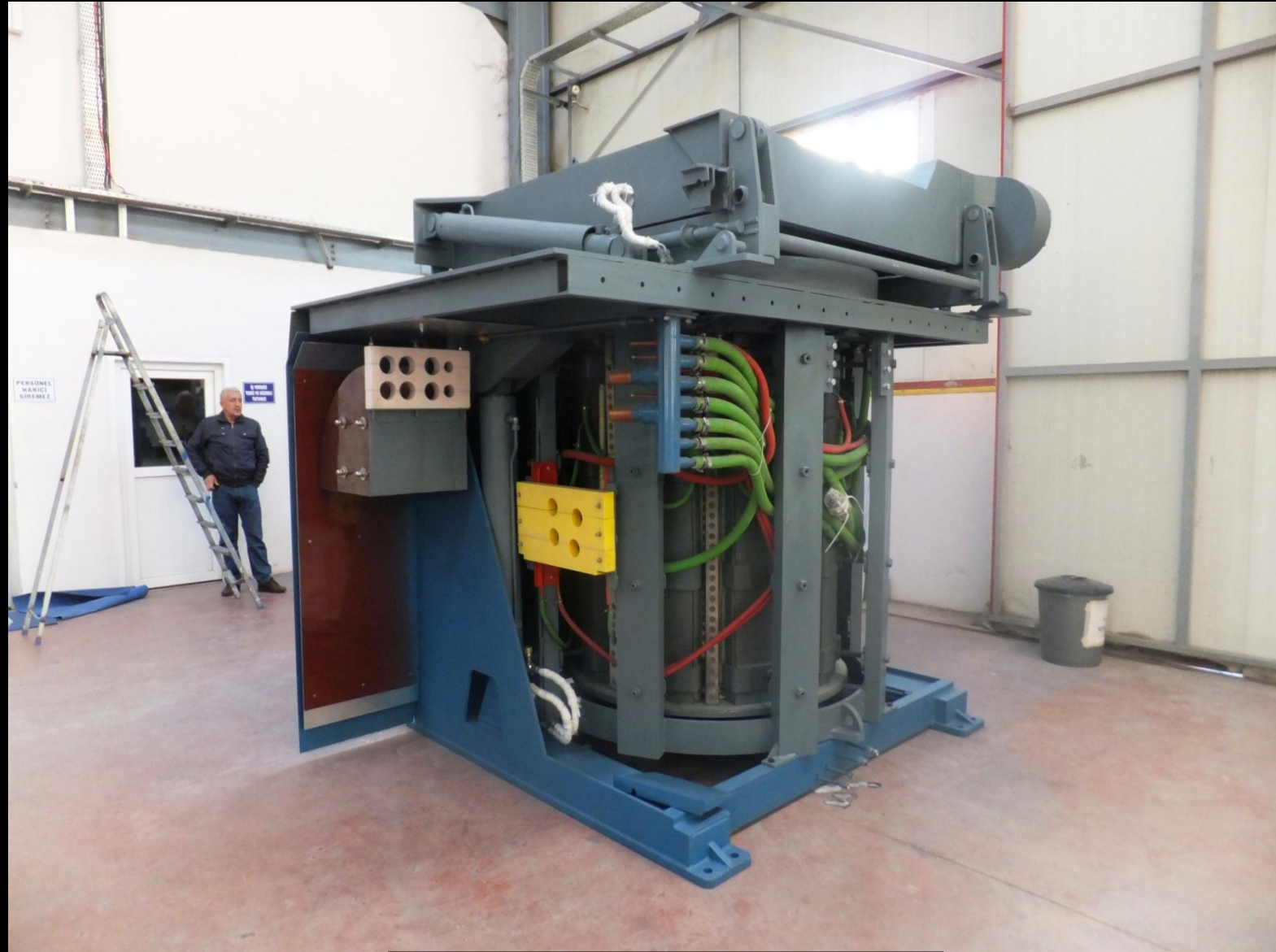
Furnace Water & Energy Connection View
